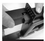
Click the letters together while standing sign on end. The Hang Tab is now fully captured on the top rail. Screw the letters together to complete sign assembly.
