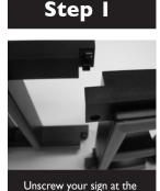
Unscrew your sign at the location(s) you've chosen to install the center support(s). Leave the rest of your sign fully assembled.
